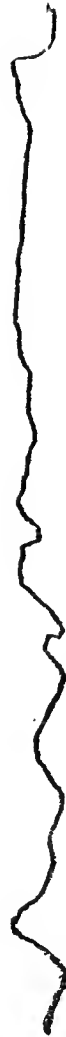
Camera lucida tracing of a machine-drawn line. Hollow of pen turned towards right. Pressure heavy. (r. h.) Magnification, 120 diameters.
