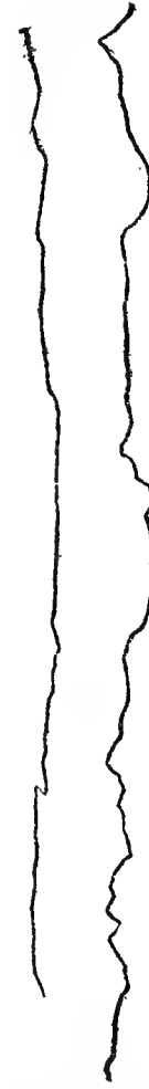
Camera lucida tracing of a machine-drawn line. Hollow of pen turned towards left. Pressure light. (l. l.) Magnification, 120 diameters.
