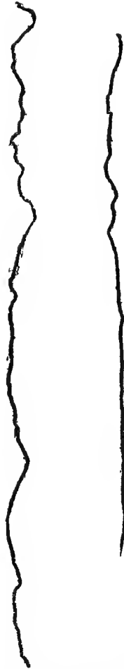
Camera lucida tracing of a machine-drawn line. Hollow of pen turned towards right. Pressure light. (r. l.) Magnification, 120 diameters.
